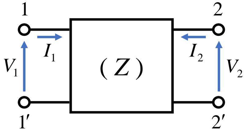
$$\begin{cases} V_1 = z_{11}I_1 + z_{12}I_2 \\ V_2 = z_{21}I_1 + z_{22}I_2 \end{cases} \Rightarrow \begin{bmatrix} V_1 \\ V_2 \end{bmatrix} = \begin{bmatrix} z_{11} & z_{12} \\ z_{21} & z_{22} \end{bmatrix} \begin{bmatrix} I_1 \\ I_2 \end{bmatrix}$$
