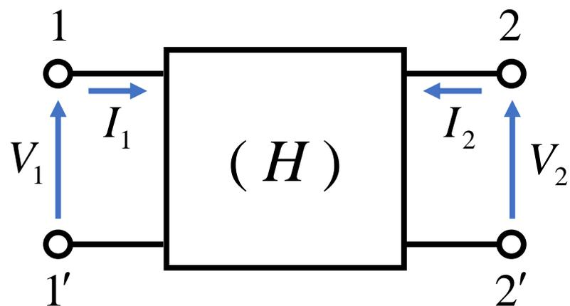
$$\begin{cases} V_1 = h_{11}I_1 + h_{12}V_2 \\ I_2 = h_{21}I_1 + h_{22}V_2 \end{cases} \Rightarrow \begin{bmatrix} V_1 \\ I_2 \end{bmatrix} = \begin{bmatrix} h_{11} & h_{12} \\ h_{21} & h_{22} \end{bmatrix} \begin{bmatrix} I_1 \\ V_2 \end{bmatrix}$$
