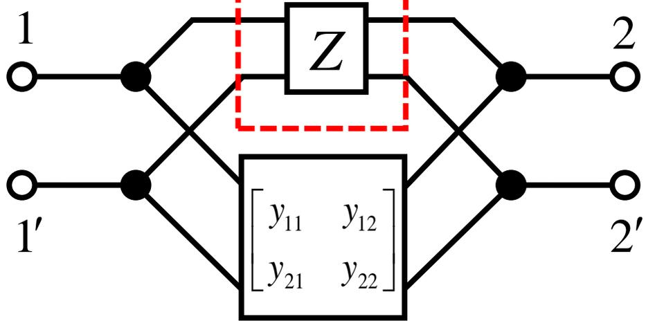
$$[Y] = \begin{bmatrix} y_{11} & y_{12} \\ y_{21} & y_{22} \end{bmatrix} + \begin{bmatrix} \frac{1}{Z} & -\frac{1}{Z} \\ -\frac{1}{Z} & \frac{1}{Z} \end{bmatrix} = \begin{bmatrix} y_{11} + \frac{1}{Z} & y_{12} - \frac{1}{Z} \\ y_{21} - \frac{1}{Z} & y_{22} + \frac{1}{Z} \end{bmatrix}$$
