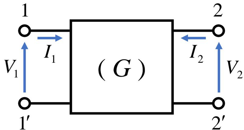
$$\begin{cases} I_1 = g_{11}V_1 + g_{12}I_2 \\ V_2 = g_{21}V_1 + g_{22}I_2 \end{cases} \Rightarrow \begin{bmatrix} I_1 \\ V_2 \end{bmatrix} = \begin{bmatrix} g_{11} & g_{12} \\ g_{21} & g_{22} \end{bmatrix} \begin{bmatrix} V_1 \\ I_2 \end{bmatrix}$$
