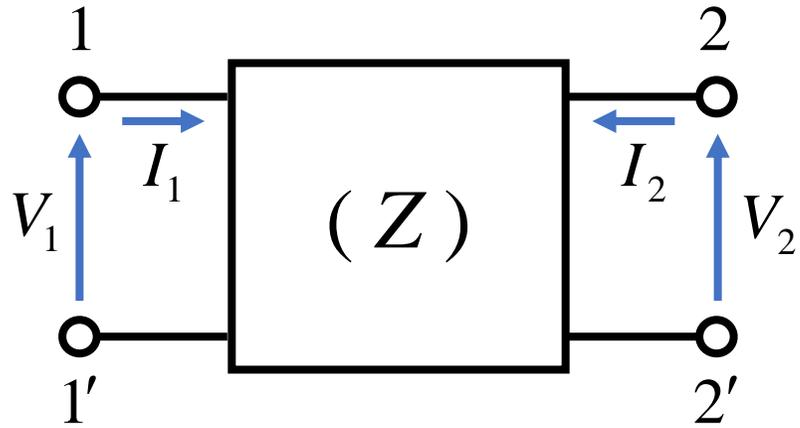
$$\begin{cases} V_1 = z_{11}I_1 + z_{12}I_2 \\ V_2 = z_{21}I_1 + z_{22}I_2 \end{cases} \quad \rightarrow \quad \begin{bmatrix} V_1 \\ V_2 \end{bmatrix} = \begin{bmatrix} z_{11} & z_{12} \\ z_{21} & z_{22} \end{bmatrix} \begin{bmatrix} I_1 \\ I_2 \end{bmatrix}$$
