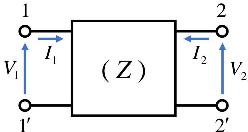
$$\begin{cases} V_1 = z_{11}I_1 + z_{12}I_2 \\ V_2 = z_{21}I_1 + z_{22}I_2 \end{cases} \Rightarrow \begin{bmatrix} V_1 \\ V_2 \end{bmatrix} = \begin{bmatrix} z_{11} & z_{12} \\ z_{21} & z_{22} \end{bmatrix} \begin{bmatrix} I_1 \\ I_2 \end{bmatrix}$$
