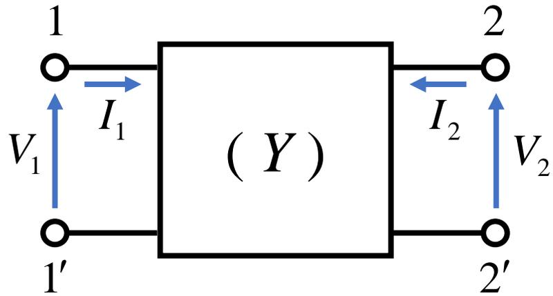
$$\begin{cases} I_1 = y_{11}V_1 + y_{12}V_2 \\ I_2 = y_{21}V_1 + y_{22}V_2 \end{cases} \Rightarrow \begin{bmatrix} I_1 \\ I_2 \end{bmatrix} = \begin{bmatrix} y_{11} & y_{12} \\ y_{21} & y_{22} \end{bmatrix} \begin{bmatrix} V_1 \\ V_2 \end{bmatrix}$$
