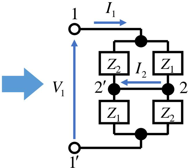
$$y_{11} = \left. \frac{I_1}{V_1} \right|_{V_2=0} = \frac{Z_1 + Z_2}{2Z_1Z_2} = y_{22}$$
