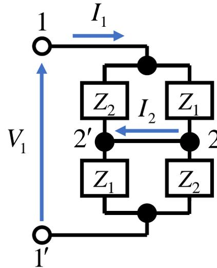
$$B = \left. \frac{V_1}{I_2} \right|_{V_2=0} = \frac{V_1}{\frac{Z_2 - Z_1}{2Z_1Z_2} V_1} = \frac{2Z_1Z_2}{Z_2 - Z_1}$$
