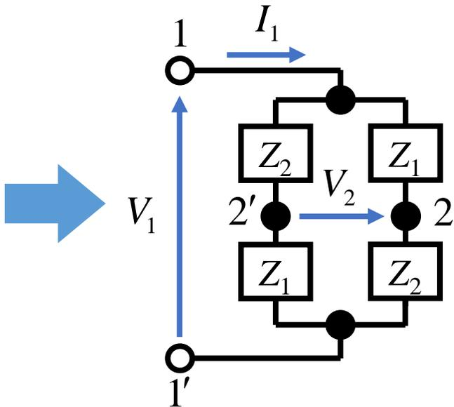
$$z_{11} = \frac{V_1}{I_1} \Big|_{I_2=0} = \frac{Z_1 + Z_2}{2} = z_{22}$$
