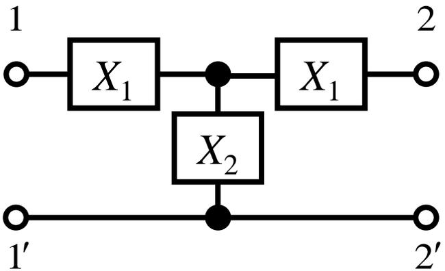
$$\begin{bmatrix} A & B \\ C & D \end{bmatrix} = \begin{bmatrix} 1 + \frac{X_1}{X_2} & 2X_1 + \frac{X_1^2}{X_2} \\ \frac{1}{X_2} & 1 + \frac{X_1}{X_2} \end{bmatrix}$$
