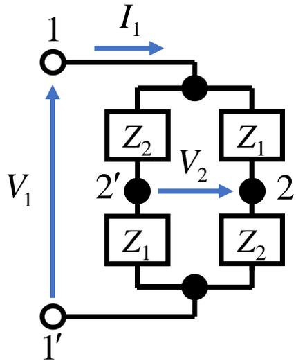
$$A = \left. \frac{V_1}{V_2} \right|_{I_2=0} = \frac{V_1}{\frac{Z_2 - Z_1}{Z_1 + Z_2} V_1} = \frac{Z_1 + Z_2}{Z_2 - Z_1}$$
