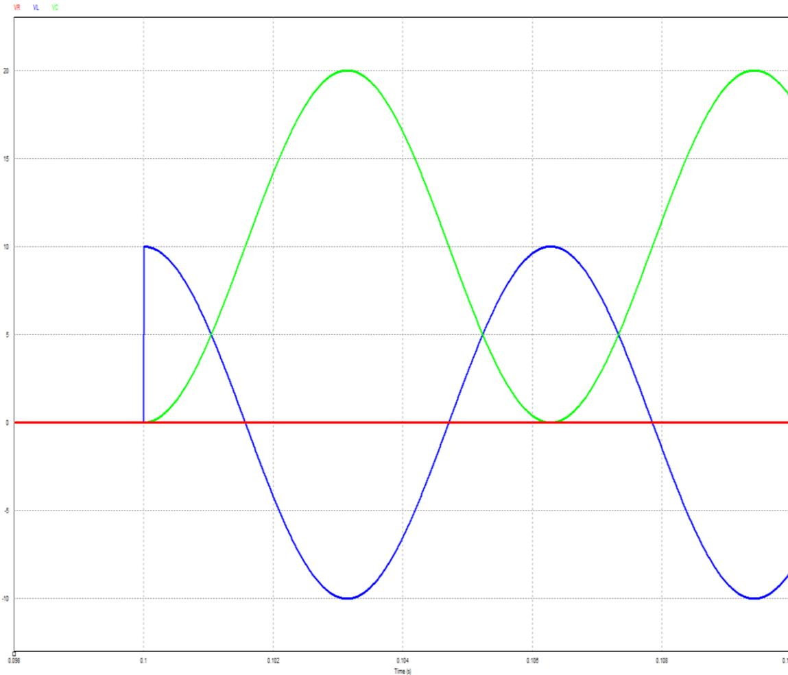
$V = 10[\text{V}]$ ,  $R = 0[\Omega]$ ,  $L = 10[\text{mH}]$ ,  $C = 10[\text{mF}]$ ,
