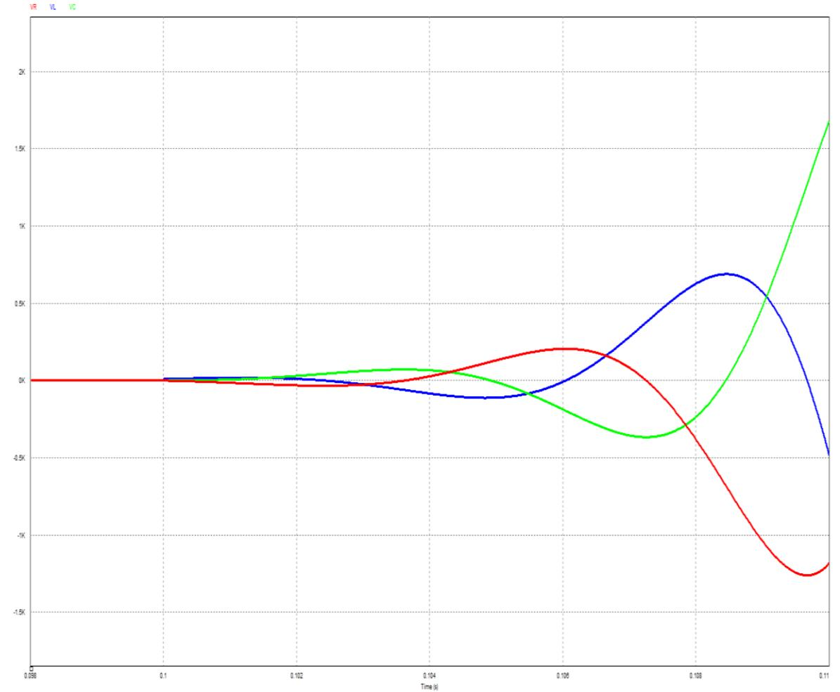
$V = 10[\text{V}]$ ,  $R = -1[\Omega]$ ,  $L = 10[\text{mH}]$ ,  $C = 10[\text{mF}]$ ,
