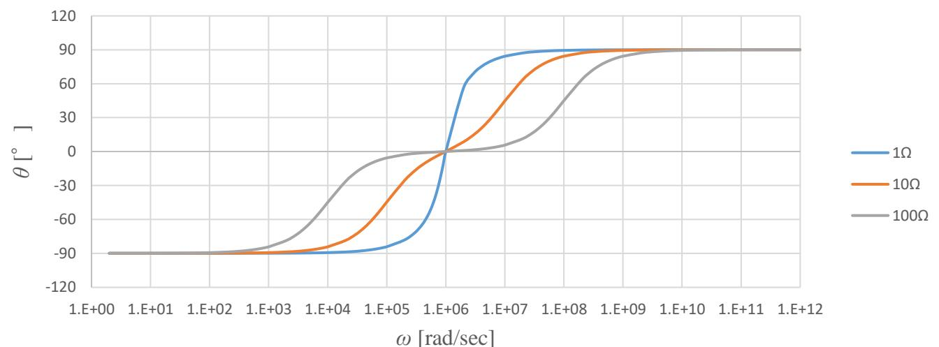
$R : 1[\Omega], 10[\Omega], 100[\Omega], L : 1[\mu\text{H}], C : 1[\mu\text{F}]$
